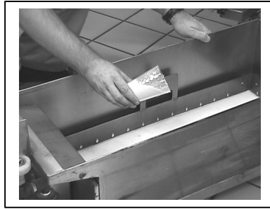
8. Sprinkle 16oz of filter powder onto filter paper in filter pan. Make sure top filter sheet is covered evenly.
